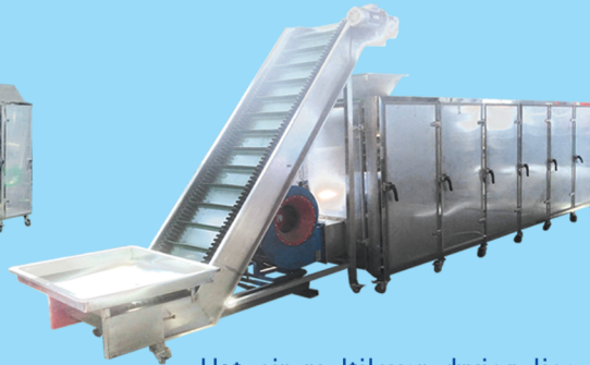
Hot air multilayer drying line
