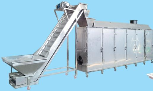
Natural wind multi-layer air drying assembly line
